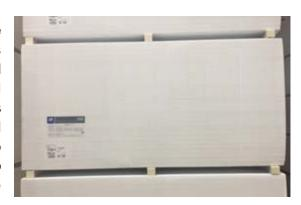
• Plastic Bag Packaging is shipped to the job site without tarps as this packaging protects the insulation during shipment. For storage less than 2 weeks, the packaging is adequate for outside storage without tarps provided the insulation arrives intact with the original undamaged weather-tight plastic bag. For storage greater than 2 weeks, JM recommends slitting the plastic shrink bag prior to
